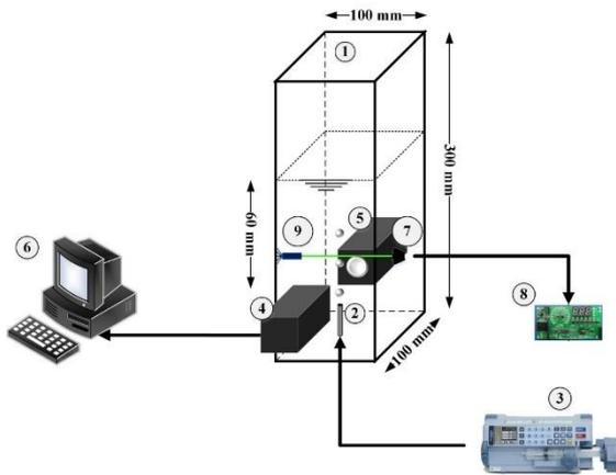
**Fig. 1.** Schematic view of the experimental setup: (1) bubble column (2) injection needle (3) syringe pump (4) high-speed video camera (5) light source (6) computer (7) phototransistor (8) electronic board (9) laser
