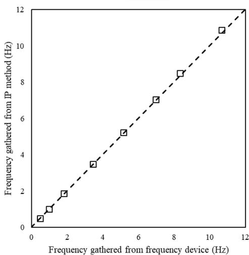
Fig. 7. Frequency of bubble formation from IP method versus frequency device method
