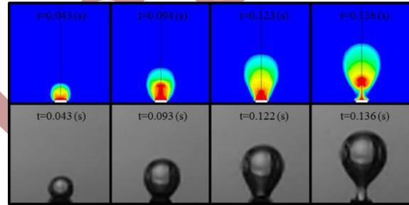
Fig. 5. Comparison of bubble formation sequence between numerical and experimental data for 800 ml/hr flow rate
