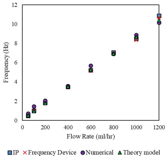
Fig. 6. Frequency of bubble formation versus flow rate for four methods
