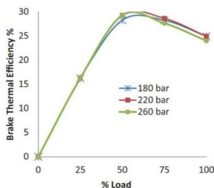
**Fig. 5. Brake thermal efficiency vs Engine load at different injection pressures**
