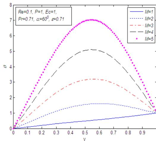
Fig. 7: Temperature field for different values of the Hartmann number  $M$
