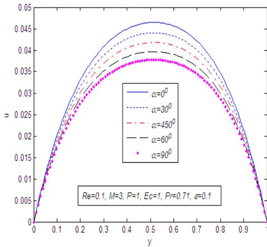
Fig. 3: Velocity profiles for different inclination angle  $\alpha$
