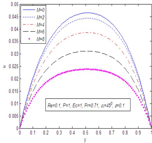
Fig. 2: Velocity profiles for different values of the Hartmann number  $M$
