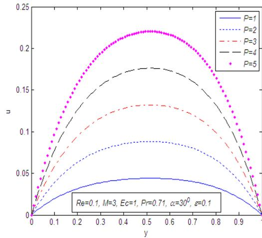
Fig. 5: Velocity profiles for different values of the dimensionless pressure gradient  $P$
