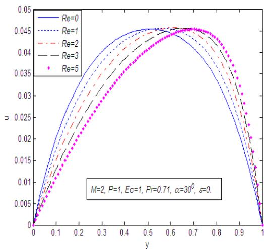
Fig. 4: Velocity profiles for different values of the suction Reynolds number  $Re$
