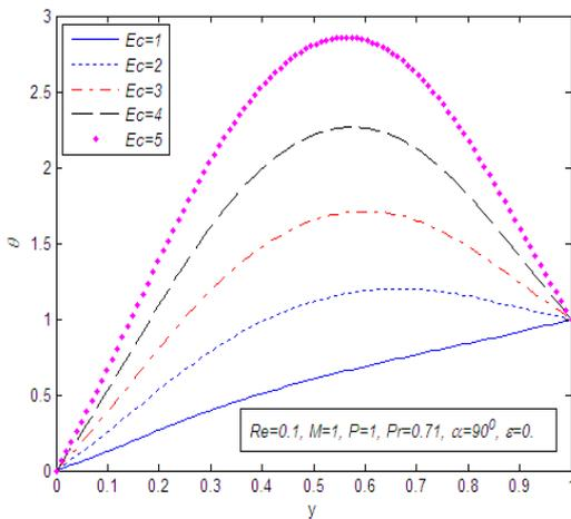
**Fig. 9:** Temperature field for different values of the Eckert number  $Ec$
