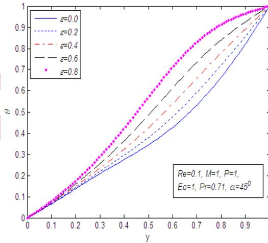
Fig. 6: Temperature field for different values of the variable thermal conductivity  $\epsilon$
