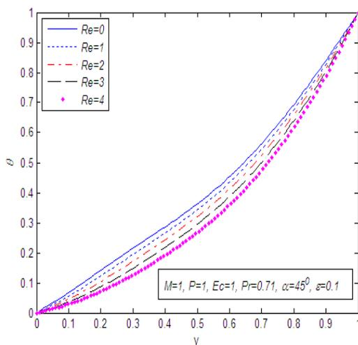
**Fig. 10:** Temperature field for different values of the suction Reynolds number  $Re$
