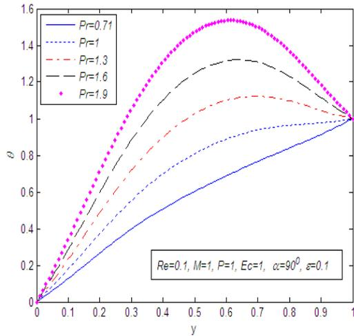
**Fig. 8:** Temperature field for different values of the Prandtl number  $Pr$
