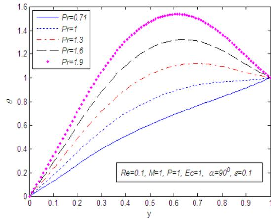
**Fig. 8.** Temperature field for different values of the Prandtl number  $Pr$
