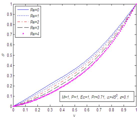
**Fig. 10.** Temperature field for different values of the suction Reynolds number  $Re$
