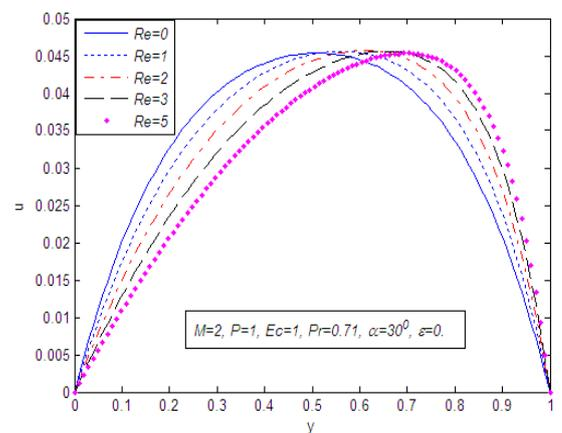
Fig. 4. Velocity profiles for different values of the suction Reynolds number  $Re$ .
