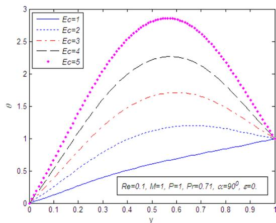
**Fig. 9.** Temperature field for different values of the Eckert number  $Ec$
