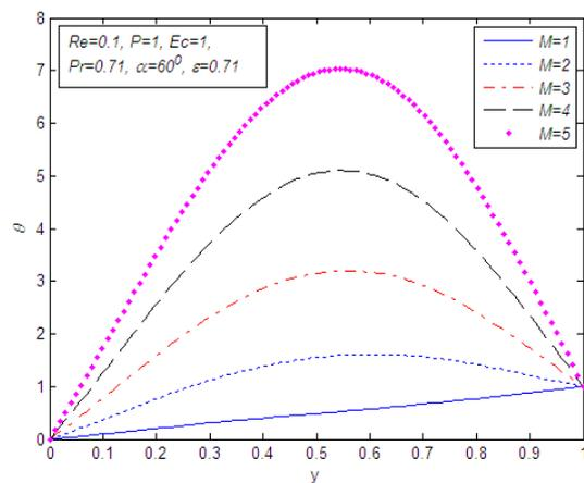
**Fig. 7.** Temperature field for different values of the Hartmann number  $M$ .
