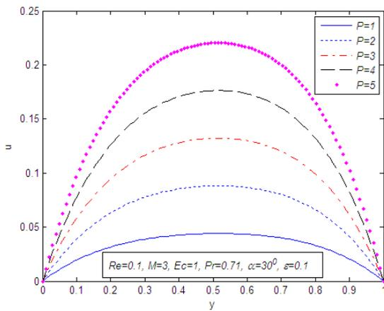
**Fig. 5.** Velocity profiles for different values of the dimensionless pressure gradient  $P$ .
