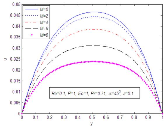
Fig. 2. Velocity profiles for different values of the Hartmann number  $M$ .
