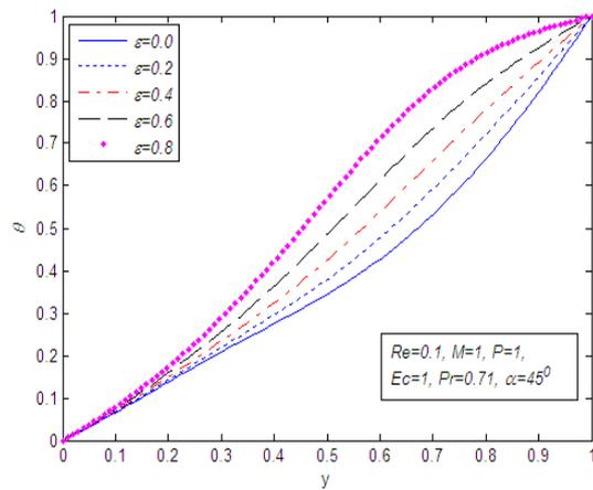
**Fig. 6.** Temperature field for different values of the variable thermal conductivity  $\epsilon$ .
