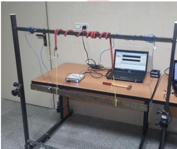
Fig. 2. Setup of OMA test.
