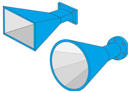
Figure 1: Conventional pyramidal and conical horn antennas.
