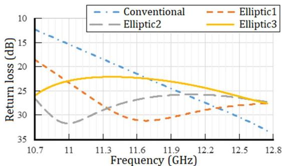
Figure 5: Comparison of the return loss of the proposed antenna with the conventional axial corrugated horn antenna.
