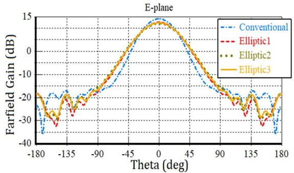
Figure 10: Optimized E-plane far-field radiation patterns for the proposed and the conventional axial corrugated horn antennas.
