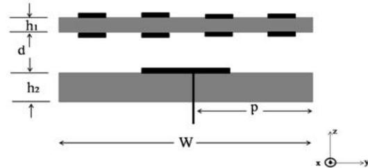
Figure 6: Side view of microstrip patch antenna covered by the metamaterial superstrate.
