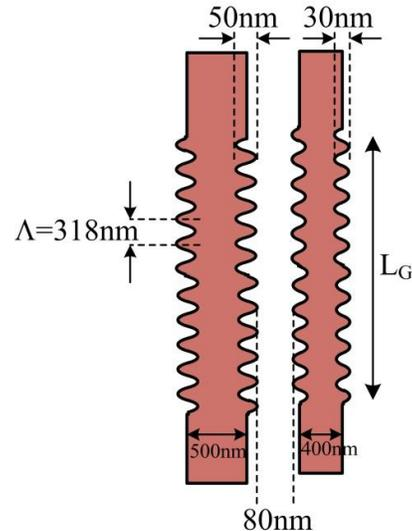
Figure 3: The Bragg grating and its structural parameters.
