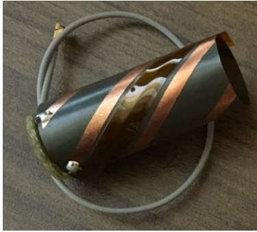
Figure 8: Fabricated antenna integrated with the feed network.
