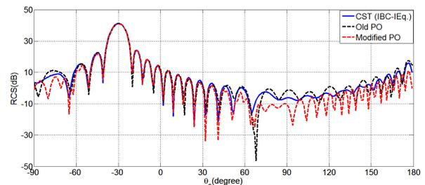
Figure 15: Bistatic RCS for the coated PEC cone in elevation plane that  $\theta_i = 30^\circ$ ,  $\phi_i = 0^\circ$  and  $\phi_s = 0^\circ$ .
