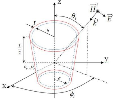
Figure 6: The geometry of the finite cone scatterer.
