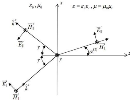
Figure 3: Incident, reflected and transmitted fields into the dielectric layer for parallel polarization case.
