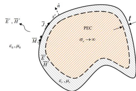
Figure 2: Induced currents at the boundary of a coated PEC object.
