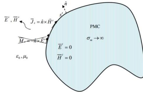
Figure 5: Zero field inside the dielectric coated object and remove one of the surface currents with filling it by PMC.
