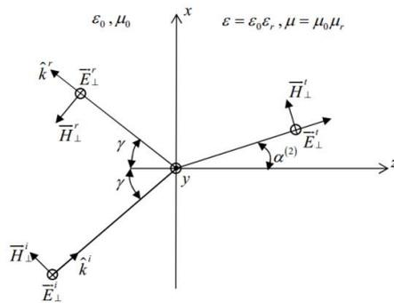
Figure 4: Incident, reflected and transmitted fields into the dielectric layer for perpendicular polarization case.
