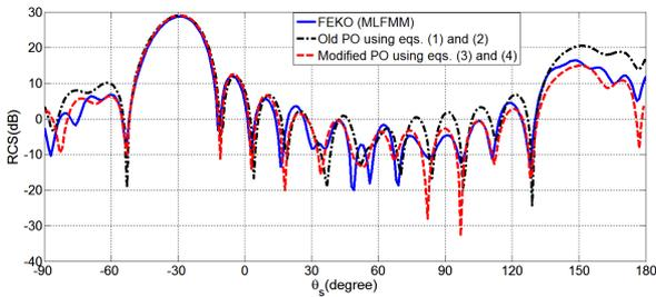
Figure 11: Bistatic RCS for the coated PEC cylinder in elevation plane that  $\theta_i = 30^\circ$ ,  $\phi_i = 0^\circ$  and  $\phi_s = 0^\circ$ .
