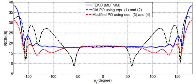
Figure 14: Bistatic RCS for the coated PEC cylinder in azimuth plane that  $\theta_i = 45^\circ$ ,  $\phi_i = 0^\circ$  and  $\theta_s = 90^\circ$ .
