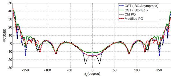
Figure 16: Bistatic RCS for the coated PEC cone in azimuth plane that  $\theta_i = 90^\circ$ ,  $\phi_i = 0^\circ$  and  $\theta_s = 90^\circ$ .
