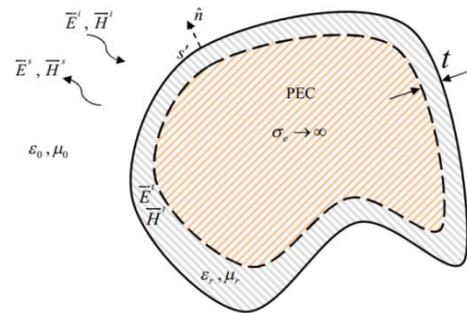
Figure 1: Incidence and reflection from a coated PEC objects.
