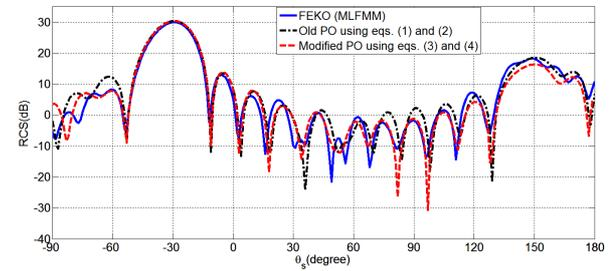
Figure 9: Bistatic RCS for the coated PEC cylinder (low-loss) in elevation plane with  $\theta_i = 30^\circ$ ,  $\phi_i = 0^\circ$  and  $\phi_s = 0^\circ$ .
