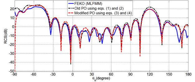
Figure 13: Bistatic RCS for the coated PEC cylinder in elevation plane that  $\theta_i = 60^\circ$ ,  $\phi_i = 0^\circ$  and  $\phi_s = 0^\circ$ .
