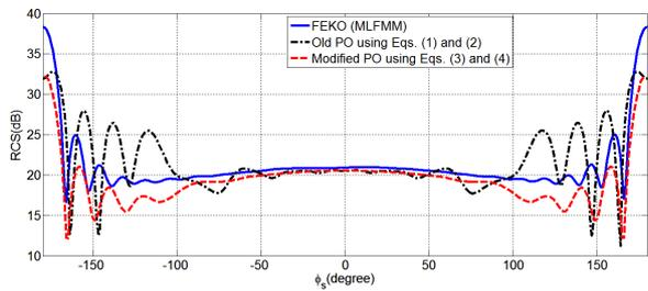
Figure 12: Bistatic RCS for the coated PEC cylinder in azimuth plane that  $\theta_i = 90^\circ$ ,  $\phi_i = 0^\circ$  and  $\theta_s = 90^\circ$ .
