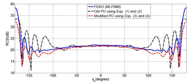
Figure 10: Bistatic RCS for the coated PEC cylinder (low-loss) in azimuth plane with  $\theta_i = 90^\circ$ ,  $\phi_i = 0^\circ$  and  $\theta_s = 90^\circ$ .
