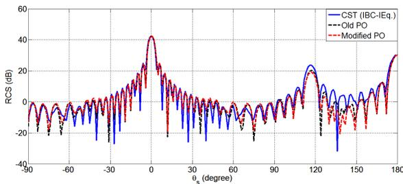
Figure 17: Monostatic RCS for the coated PEC cone at  $\phi_i = 0^\circ$  and  $\phi_s = 0^\circ$  plane.
