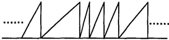
Figure 2. A randomized triangular carrier signal in RPWM modulator
