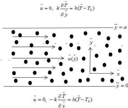
Fig 1. The formulation geometry
