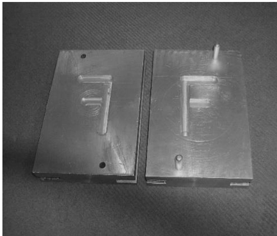
Fig. 2. An aluminum die used to produce of wax patterns under different conditions
